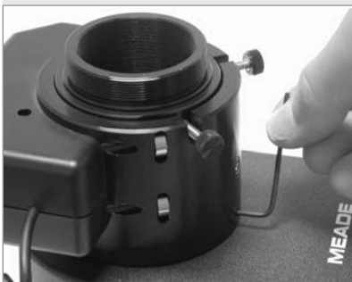
Fig. 62: Tighten the three microfocuser hex screws to a firm feel.
