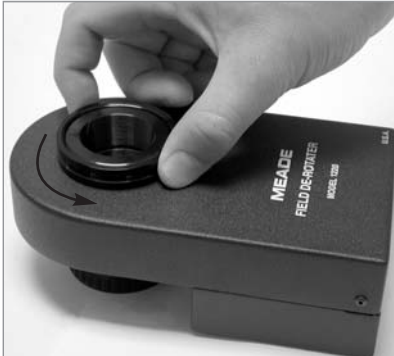
Fig. 60: Back off the adapter ring one full revolution.
