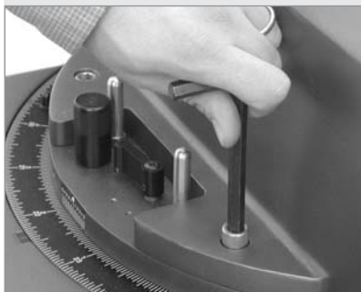
Fig. 51: Bolt the fork to the drive base.
