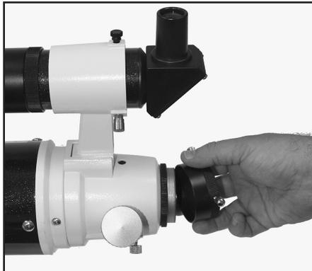
3. Remove the caps from the field flattener lens and thread it onto the focuser draw tube.
