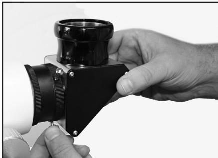
If you wish to change the orientation of the diagonal, loosen the thumb screw on the focuser draw tube. This will allow the diagonal (or camera for photography) to rotate freely. Rotate the diagonal to the desired position and tighten the screw.
