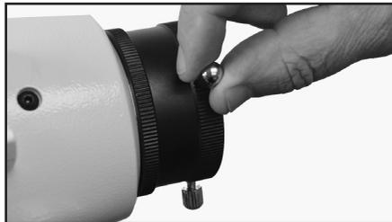
2. Slide the 2" barrel end of the diagonal into the focuser adapter ring.
