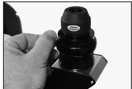
To remove the eyepiece, loosen the set screw on the diagonal and slide the eyepiece out.
