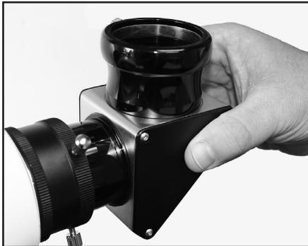
3. Tighten the set screw on the adapter ring to hold the diagonal in place.
