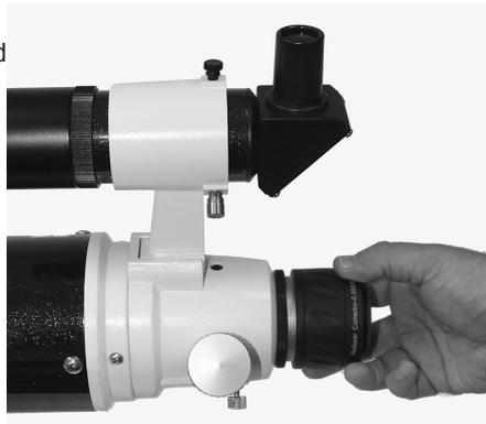
4. Now attach the M48 camera adapter onto the other end of the field flattener lens.
