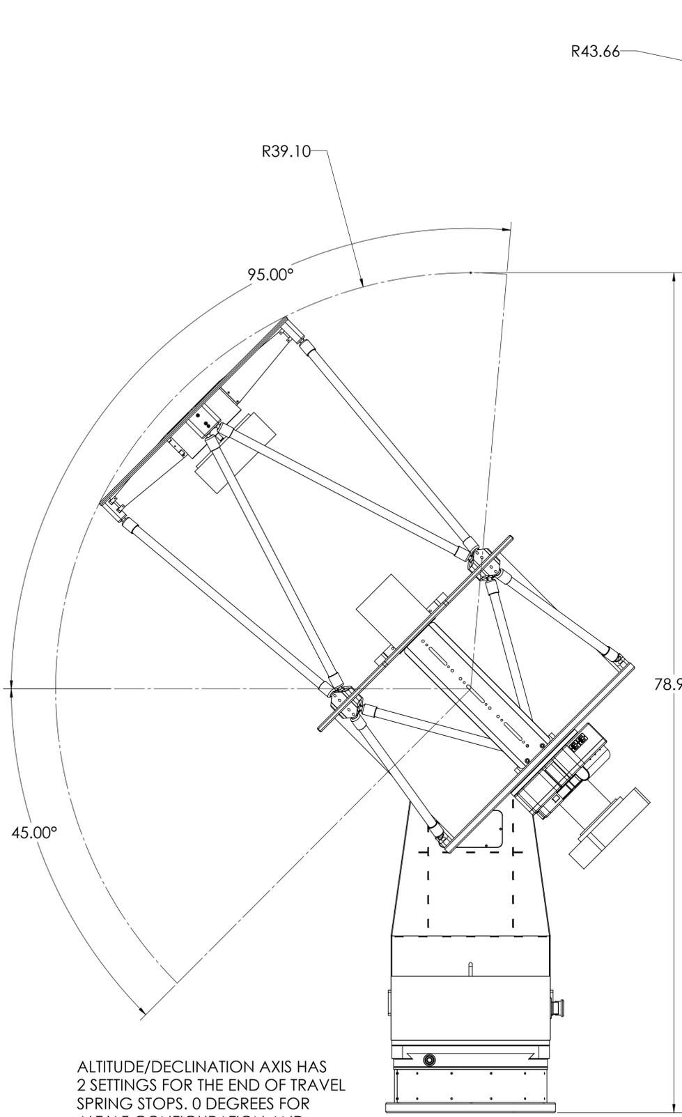
ALTITUDE/DECLINATION AXIS HAS 2 SETTINGS FOR THE END OF TRAVEL SPRING STOPS. 0 DEGREES FOR ALT/AZ CONFIGURATION AND -45 DEGREES FOR EQUATORIAL UPPER LIMIT IS FIXED AT 95 DEGREES
