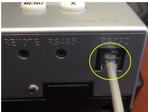
Figure 18. Connect RJ-9 cable to mount
