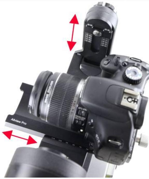
Figure 11 Adjust camera No-Parallax Point
