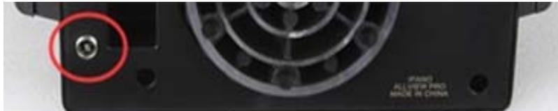
Figure 3. Direct Power Socket for 7.4V portable power pack
