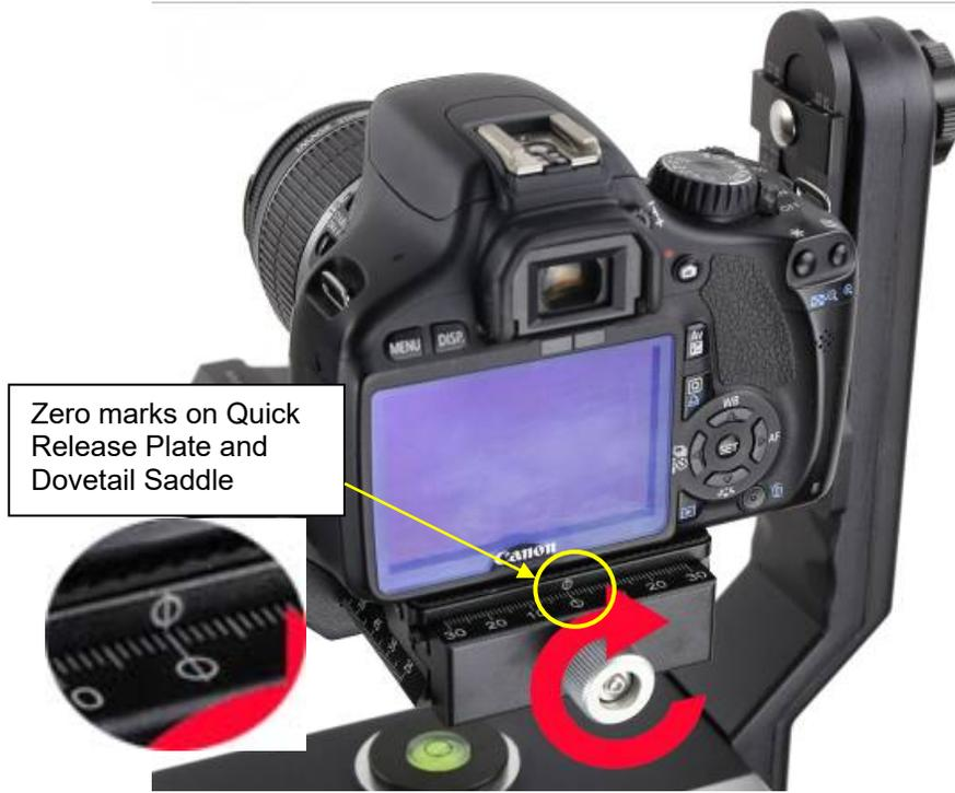
Figure 7 Align the zero marks
