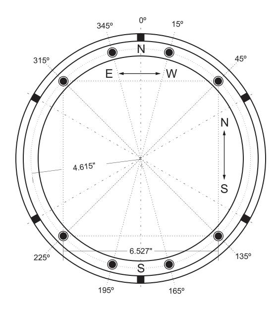
The drawing above provides the necessary detail to drill and tap your flat surface to accept the 1612FSA Flat Surface Adapter for 1200 (all versions) and 1600GTO mounts. The eight counter-bored 1/4" thru-holes are all on a 9.230" diameter bolt circle (4.615" radius).
